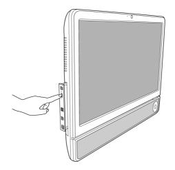
3. Pull out the disc tray and remove the disc.
